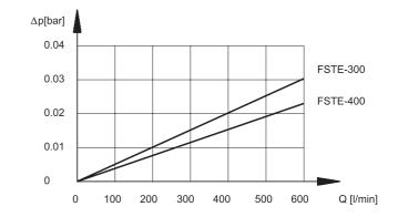
**NOTE 2:** The filter size has to be selected so that with the nominal flow rate the pressure drop is lower than 0.02 bar. The total pressure drop through the filter is given by adding the body pressure drop values to those of the filter element.
